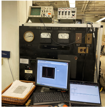
Figure 7: Set up to run the experiment. Oscilloscope and strain gauge conditioner.
