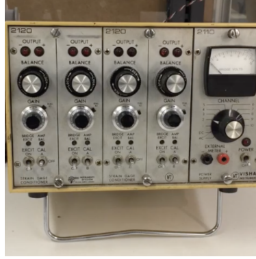
Figure 9: Vishay system used to measure drag and lift.
